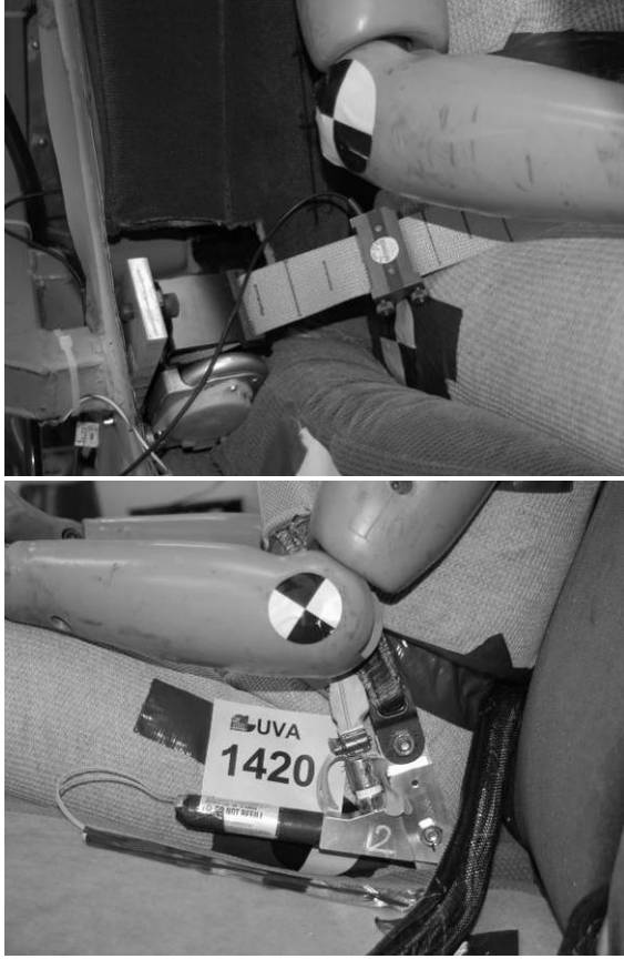
Figure 4: Close-up views of the outboard lap belt retractor (top) and the inboard assembly of the lap and shoulder belt anchors and the airbelt inflator
